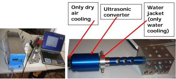
Picture of the complete ultrasonic system configuration: MMM-Generator (left), Converter-Wave-guide-Water-jacket-Aluminum block (middle) and PC (right). PC Interface RS485 to USB (or RS232) is connected between the PC and MMM generator. Client should use his own PC. Software <a href="mpi\_ix.exe">mpi\_ix.exe</a> for the MSG.1200.IX should be installed (download software here:
